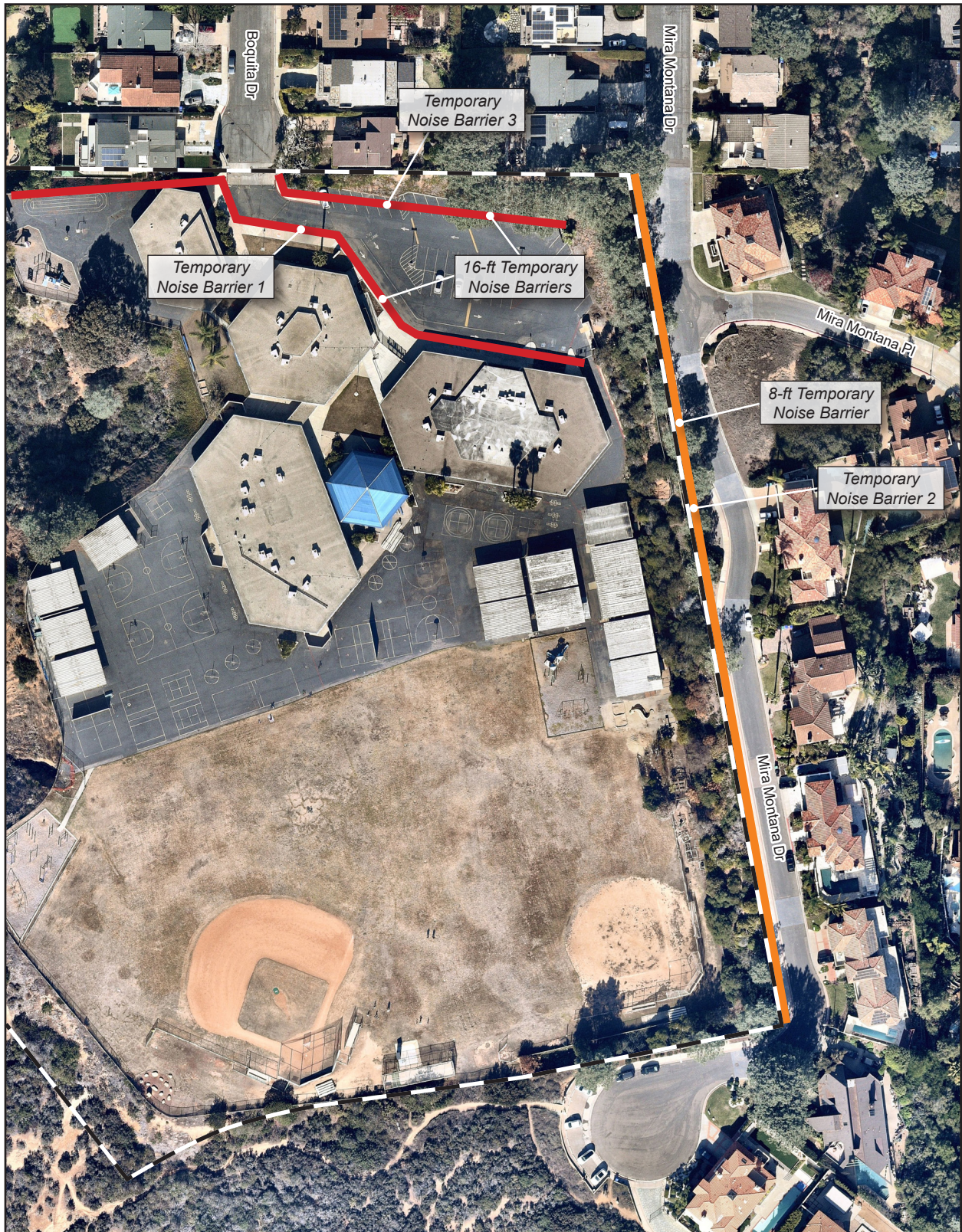
Figure 5.2-11 - Temporary Noise Barriers
