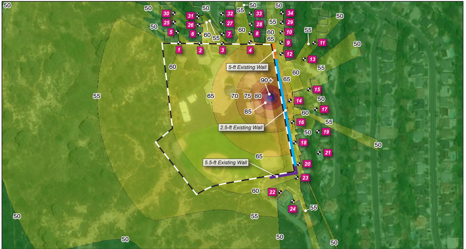
Figure 5.2-5 - Soil Nailing and Grading Center Noise Contours (Unmitigated)
